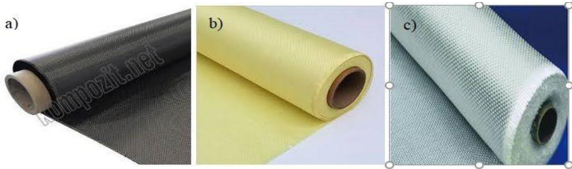
Figure 5. (a) Carbon fabric, (b) Aramid fabric, (c) Fiberglass fabric.( Soutis C, 2005.)
